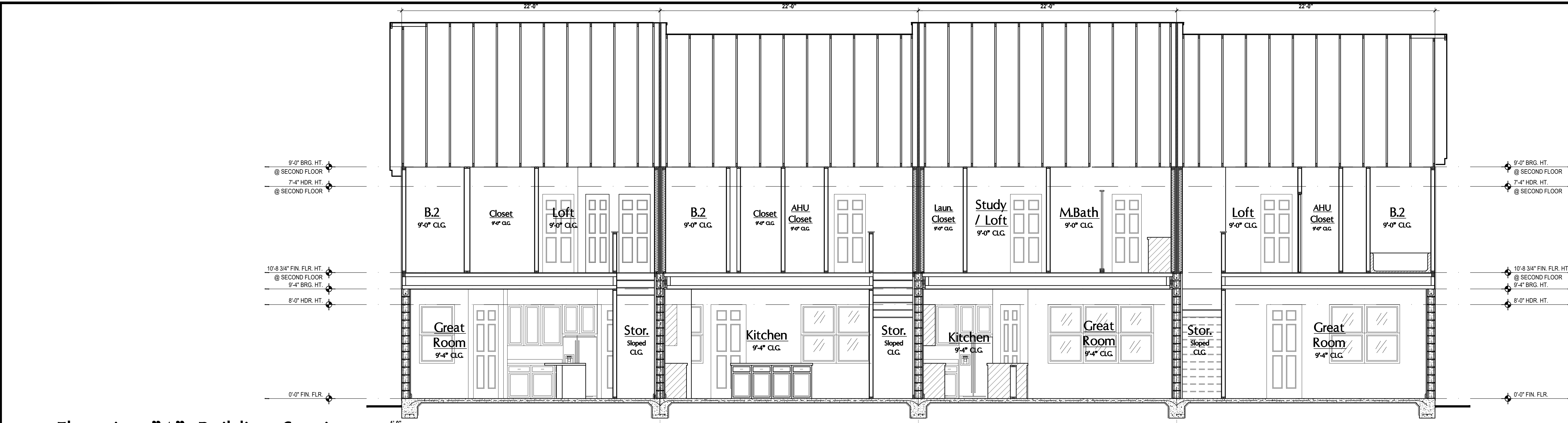
1 Elevation "A": Building Section A10 SCALE 1/4" = 1'-0"
