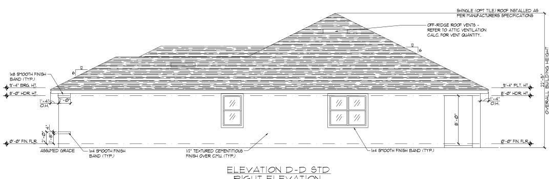
ELEVATION D-D STD RIGHT ELEVATION 1/8"=1'-Ø" (11×17) 1/4"=1'-Ø" (22×34)
